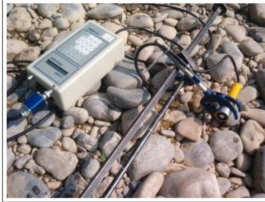
Figure 27: Light-probe and data-logger
