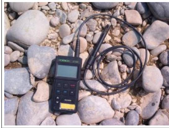
Figure 25: Conductivity meter LF323 by WTW
