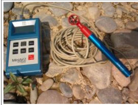
Figure 24: Velocity meter Mini-Air2 by Schiltknecht
