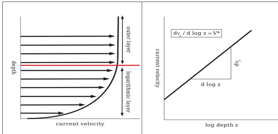
Figure 3: *Velocity - depth* and *velocity - log(depth)* diagrams with logarithmic layer
